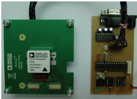
Figure 1: A photograph of the data logger system (right) and a miniature gyroscopes and accelerometers (left).
