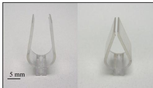
Figure 1: Shape-memory effect in an epoxy resin pincer.
