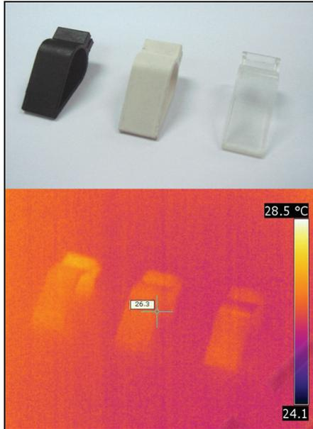
Figure 2: Importance of calibrating the emissivity of the material.
