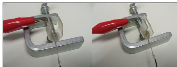
Figure 4: Activation by heating the pincer and recovery of its geometry.
