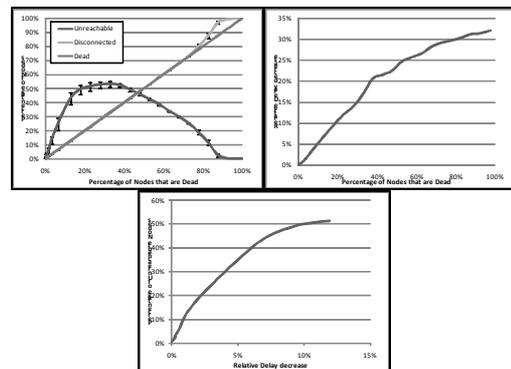
Figure 5: (a) The percentage of disconnected and unreachable nodes in the networks for varying numbers of dead nodes (1000 node topologies, 98% confidence interval). (b) The relative decrease of the end-to-end sensor to gateway delay (of the active nodes) in the networks for varying numbers of dead nodes (1000 node topologies). (c) The percentage of unreachable nodes in the network versus the relative decrease of the end-to-end delay (1000 node topologies).
