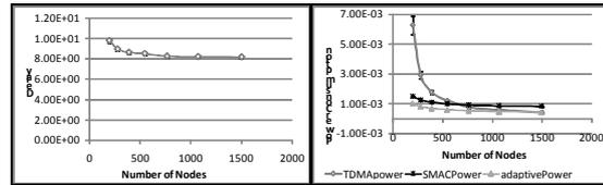
Figure 4: Delay (a) and power consumption (b) for the S-MAC, Ad\_Li, and TDMA schemes, for topologies with increasing nodes, and some traffic ( $N \lambda_0 = 0.005$ ).
