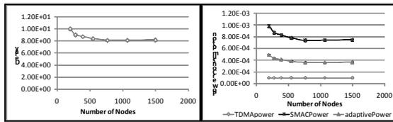
Figure 3: Delay (a) and power consumption (b) for the S-MAC, Ad\_Li and TDMA schemes, for topologies with increasing nodes, and no traffic.
