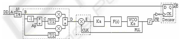
Figure 6: Analog symbol phase synchronizer.
