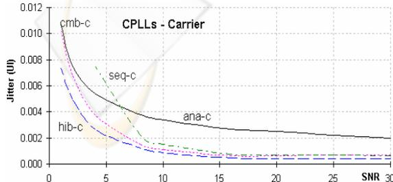
Figure 12: Jitter-SNR curves of the four carrier synchronizers (a,h,c,s).
