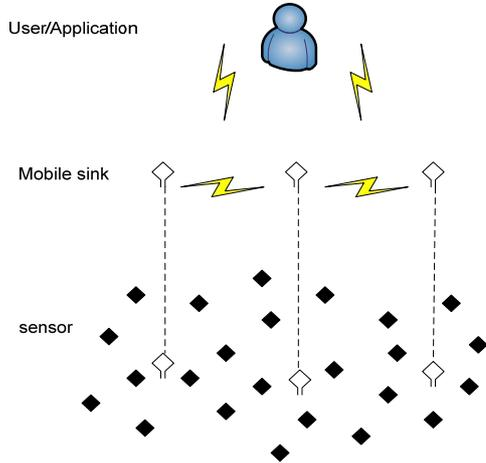
Figure 1: Architecture of a multi-tiered wireless sensor network.
