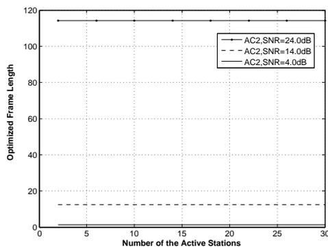
Figure 8: The optimal frame length varies with respect to the number of active stations.
