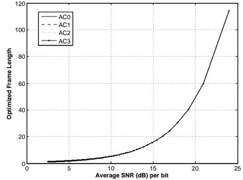
Figure 7: The optimal frame length per varies with respect to the SNR.
