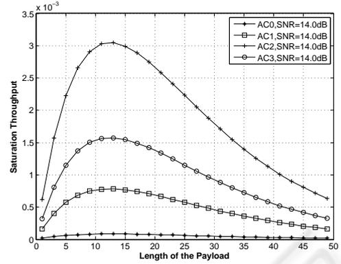
Figure 5: Saturation throughput of the ACs against the frame length (SNR=14.0dB).
