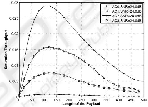
Figure 6: Saturation throughput of the ACs against the frame length (SNR=24.0dB).
