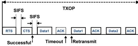
Figure 4: RTS/CTS exchange, successful transmission, retransmission and collision time.
