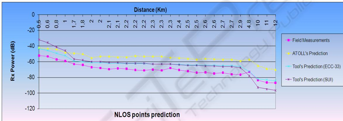
Figure 7: Comparison with measured values for NLOS areas.
