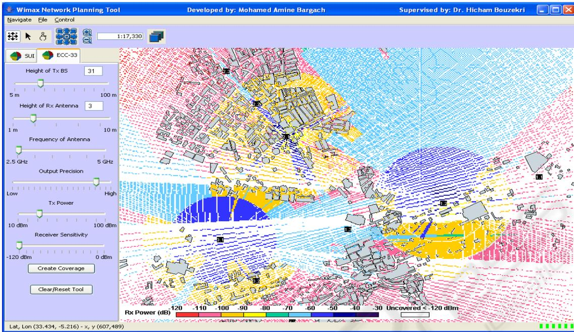
Figure 4: Optimized positions for 3 BTS.
