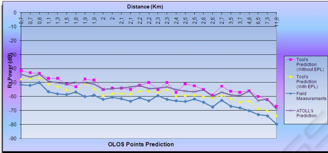
Figure 6: Comparison with measured values for OLOS areas.
