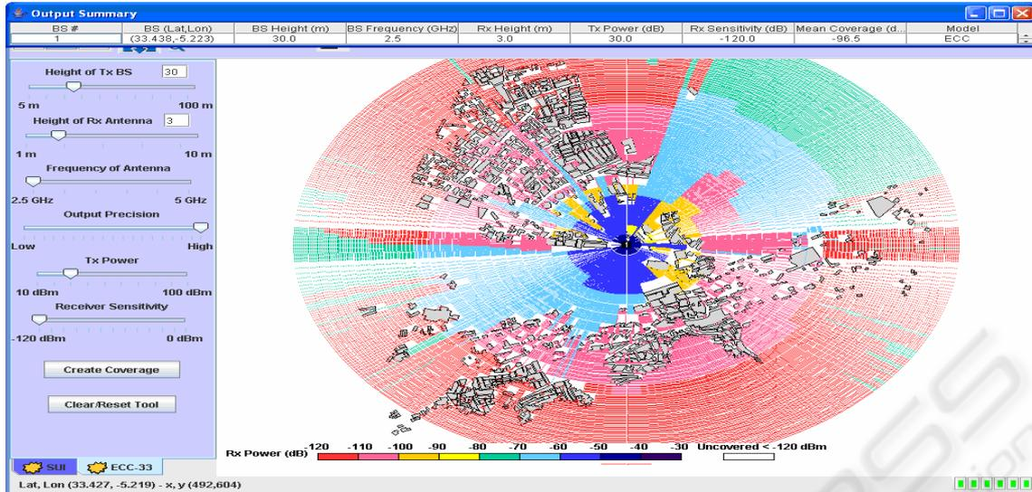
Figure 3: Predicted Coverage of the Azrou region (Normal Mode).
