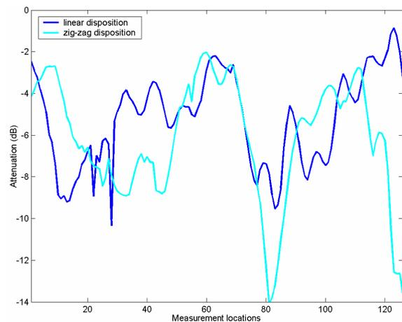
Figure 4: Median attenuation (dB) due to Irish junipers at 2.4 GHz, with horizontal polarisation.
