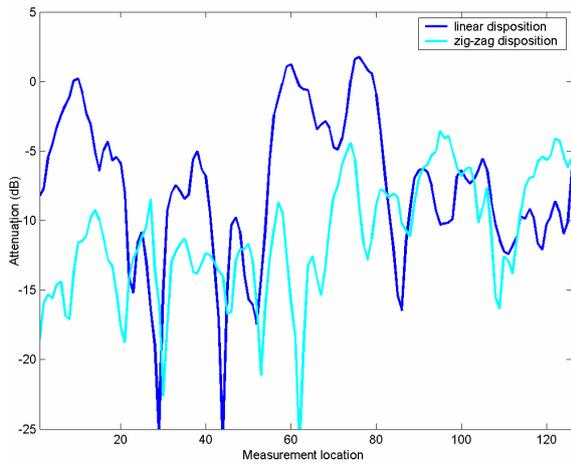
Figure 5: Median attenuation (dB) due to Irish junipers at 5.8 GHz, with horizontal polarisation.
