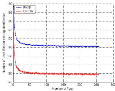
Figure 5: The number of used bits for one tag identification with the varying number of tags, PER=0.
