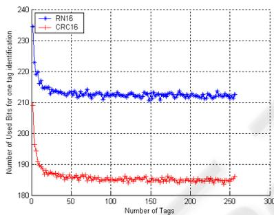
Figure 6: The number of used bits for one tag identification with the varying number of tags, PER=0.3.
