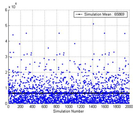
Figure 4: The uniformly random characteristics of CRC-16.
