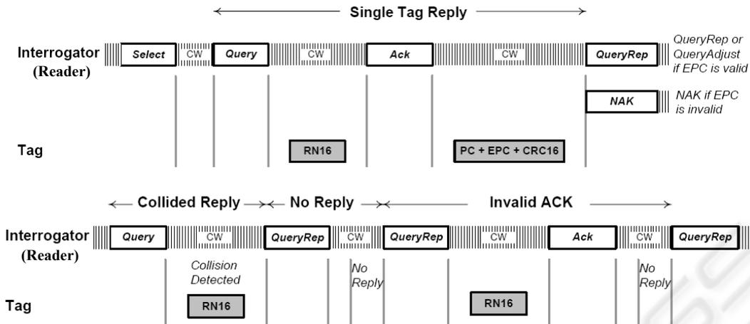
Figure 1: Tag identification mechanism using RN16 and having different time duration for success, idle, and collision.
