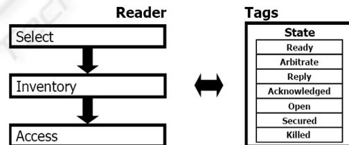
Figure 2: Reader/Tag operation and the state of tags.
