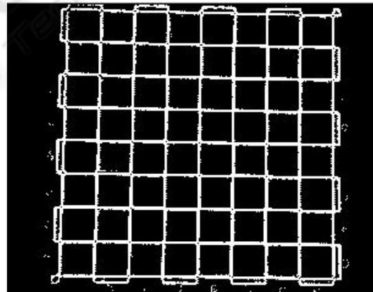
Figure 3: Recognizing the edges of the chess board.
