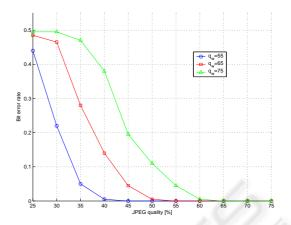
Figure 7: Robustness to JPEG compression.
