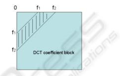
Figure 4: Frequency band for watermark embedding.
