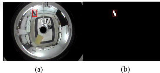
Figure 3: The results of foreground image capturing. (a) An original image; (b) A binarized image after noise removal and connected component labeling.
