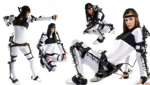
Figure 6: Mechanical motion capture system GYPSY6 made by Inition (Inition, 2008).
