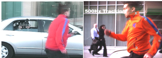
Figure 3: Prakash system, the tags are under the clothing and are activated by a multi-LED camera in the car (Raskar, 2008).
