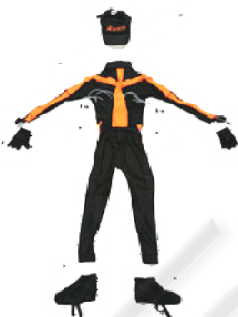
Figure 5: The suit for inertial motion capture created by MOVEN (Inition, 2008).
