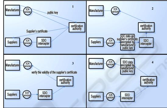
Figure 1: Process of use public/private key encryption and certificate in unsafe SOA.
