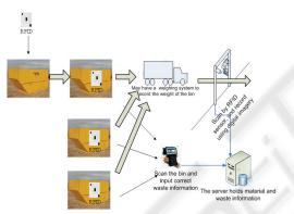
Figure 3: The Outward Material Handling System for Waste Plasterboard.
