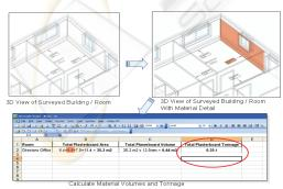
Figure 6: Predicting the Correct Volume and Tonnage of Plasterboard in Advance.
