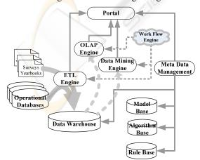
Figure 1: The Architecture of LMDSS.
