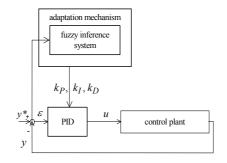
Figure 3: Block diagram of the closed-loop system with adaptation mechanism.
