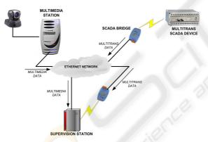
Figure 1: Ethernet SCADA bridge.
