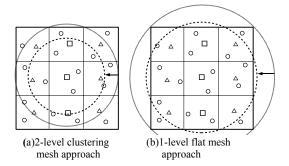
Figure 10: Restricted range in (a) 2-level clustering mesh and (b) 1-level flat mesh approaches.
