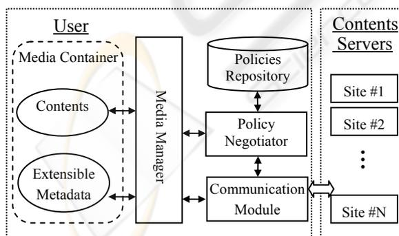
Figure 1: Functional Architecture of the Proposed Metadata System.
