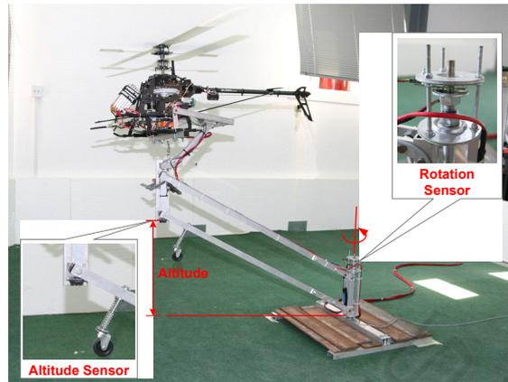
Figure 3: Positioning sensors.
