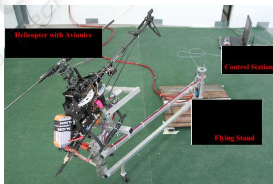
Figure 1: View of the experimental test bed.
