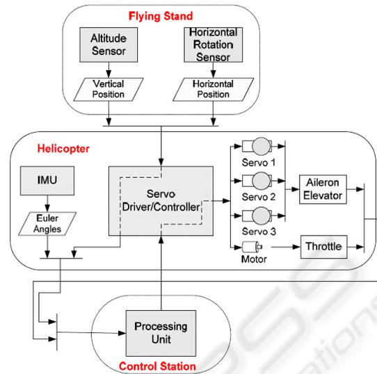
Figure 4: System Architecture.
