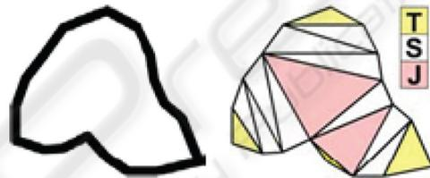
Figure 5: The triangulation strategy used by "Teddy" defines different triangles as Terminal, Sleeve or Junction depending on how many sides are shared with the silhouette.
