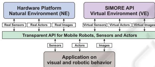
Figure 3: Transparent API provides support for real and virtual robots, sensors and actors.
