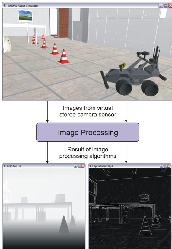
Figure 6: Stereo view of the robot's virtual camera sensor.
