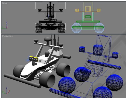
Figure 4: Modeling of collision objects in 3ds max.
