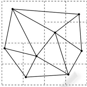
Figure 2: Example of a PM3-Triangle quadtree.
