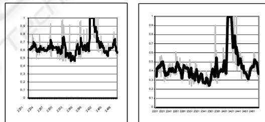
Figure 2: Left:  $P^{(U)}$  of the most suspicious blob based on the estimated probabilities for the video “Syn”. The peak at frame 2500 shows the anomalous motion. Right: using  $P^{(U,M)}$  increases the difference between the unusual event and other local peaks.
