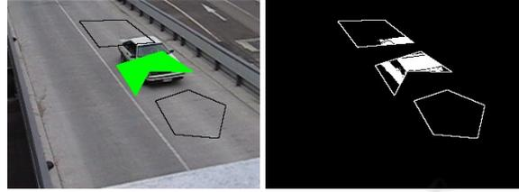
Figure 2: Sample frame and mask with polygonal sensors.
