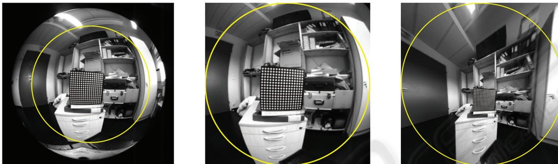
Figure 5: Correction of the radial distortion for a fish-eye lens. Left: The original fish-eye image in which the central area is denoted by the circle. Middle: The area inside the circle is transformed to the perspective model using the initial values for the internal camera parameters. The transformation is not correct since the scene lines are not straight in the image. Right: The area inside the circle is corrected using the estimated parameter values. The images of lines are straight.
