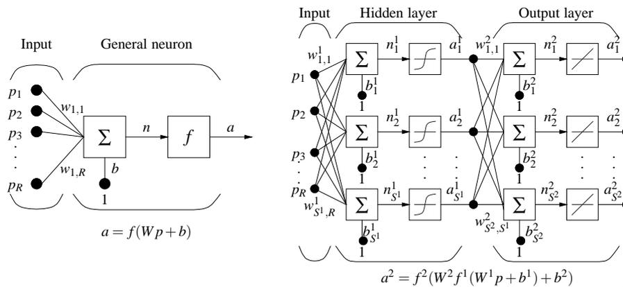
Figure 2: Neuron model and network architecture.
