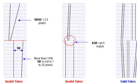
Figure 4: Determine the valid tube.
