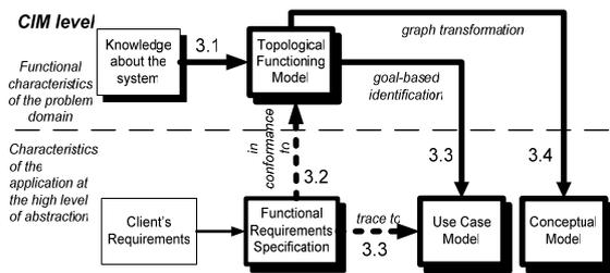
Figure 2: CIM creation with the TFMfMDA in the OOA with Separation of Concerns.
