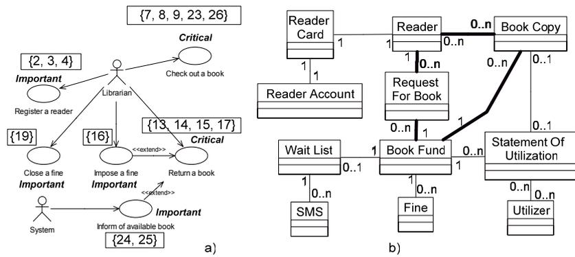
Figure 4: The use case model (a); and the initial conceptual model (b).
