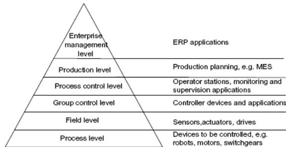
Figure 2: The overall enterprise information systems with its levels.
