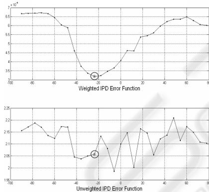
Figure 3: Weighting the Error Function clearly sharpens its minimum peak.
