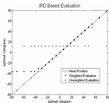
Figure 9: Localization of a narrowband signal. Results are shown for weighted ILD (stars) weighted IPD (diamonds) and unweighted IPD (crosses).
