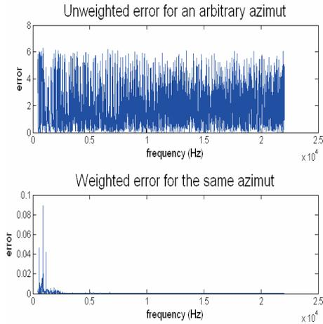
Figure 2: Unweighted and weighted error as function of the frequency for an arbitrary azimuth.
