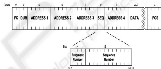
Figure 1: Format of 802.11 Frame Header (IEEE Wireless LAN Standard, n.d.).
