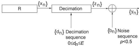
Figure 3: The statistical model of the step 1/step  $E$  generator.
