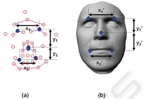
Figure 5: Illustration of calculating the scale factor to convert motion capture data into the space of the databank. (a) Neutral motion capture data; (b) Neutral model in the databank.
