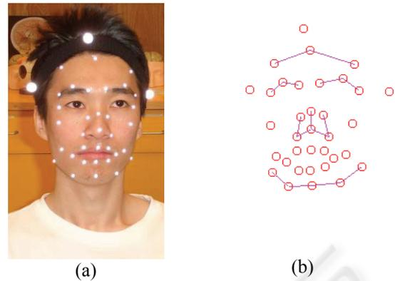
Figure 4: Facial motion capture using a *VICON™* system. (a) Sparse markers are attached to the subject's face; (b) 3D virtual markers reconstructed by the *VICON™* system.
