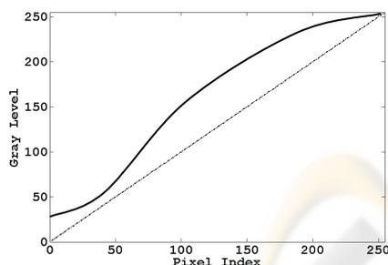
Figure 1: Straight line represents the gray levels varying linearly from 0 to 255. The curved plot represents the change in gray levels after image acquisition.
