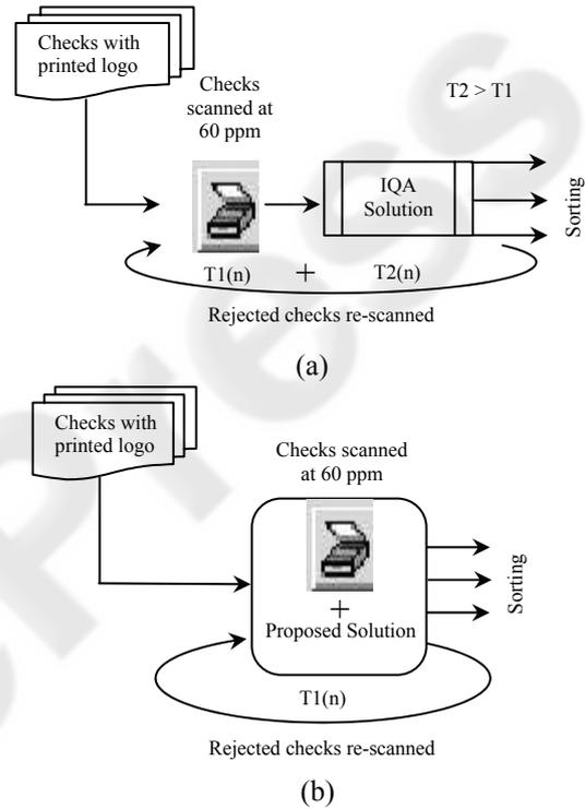
Figure 7: (a) A schematic diagram indicating the total time taken by the existing image acquisition and quality analysis phase. (b) A schematic diagram indicating the deployment of the proposed solution at the point of capture and reduction in time.
