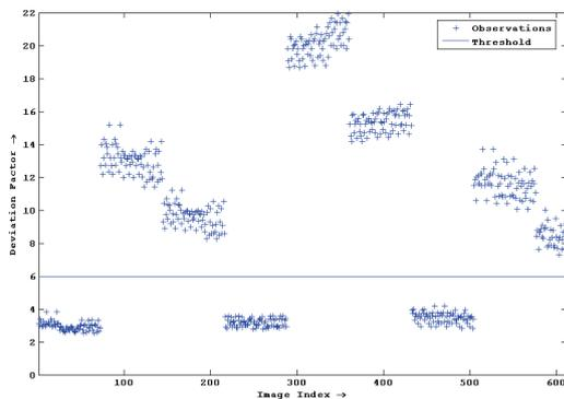
Figure 9:  $\sigma$  plotted for the data set of 612 images. Images with  $\sigma$  above the threshold have been rejected on the count of bad quality.
