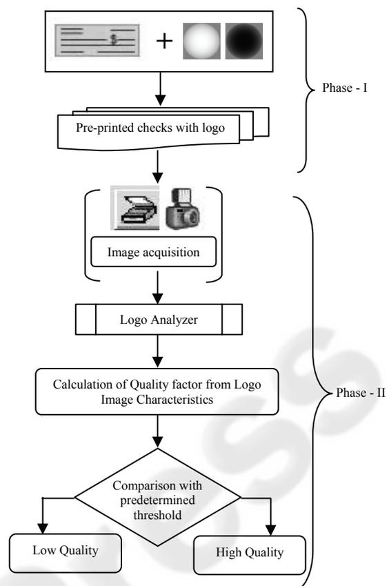
Figure 2: Block diagram of the proposed method.
