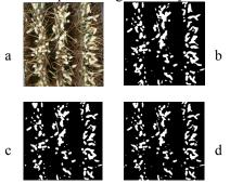
Figure 4: Results of segmentation obtained by the different techniques implemented for a whole image: (a) Test image. (b) with 1<sup>st</sup> order statistic. (c) with co-occurrence matrix. (d) with run length.
