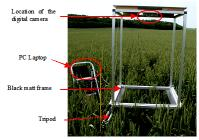
Figure 2: In Field image acquisition system.
