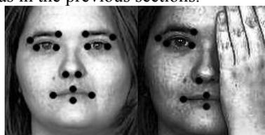
Figure 4: Image with the 14 fiducial points considered for an image with all the face features visible (left). For images with occlusions, only 8 points were taken into account (right).
