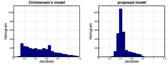
Figure 3: Circle-to-Ellipse example. Histograms of Jacobian values of the deformations inside the ellipse for Christensen's model and the proposed model.
