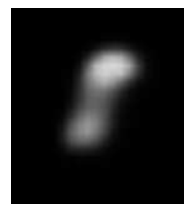
Figure 3: The Effects of Vibration on a Single Luminaire.
