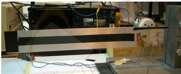
Figure 5: The smart beam used in the study.
