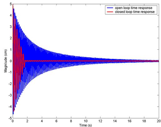
Figure 7: Free vibration suppression of the smart beam.
