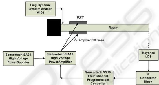
Figure 6: The closed loop experimental setup.
