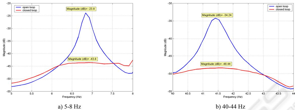
Figure 8: Bode magnitude plot of the open and closed loop systems.
