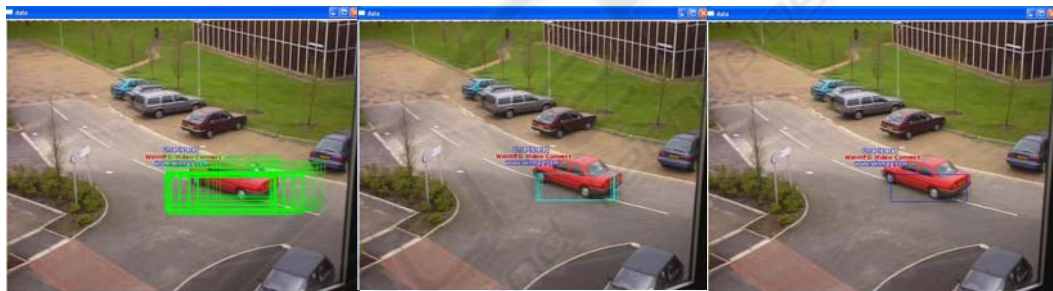
Figure 3: Tracking procedure using PSO-based searching.
