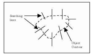
Figure 5: Normal lines of object contour to search the observation  $z_i$ .
