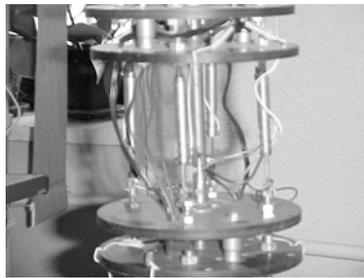
Figure 1: The proposed SMA robotic ankle.
