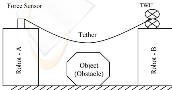
Figure 3: Schematic of Experimental Setup.
