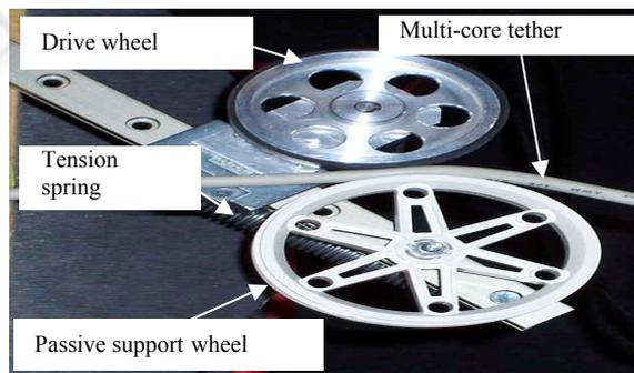
Figure 1: Tether Winding Unit (TWU).
