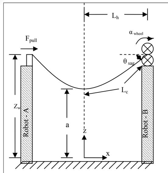
Figure 5: Tether Entanglement Detections System (TEDS) Model.
