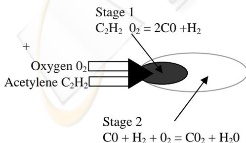
Figure 13: Oxy-Acetylene flame.
