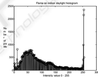
Figure 8: Flame on daylight histogram.
