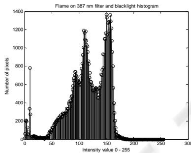
Figure 10: Flame on 387 nm image histogram.
