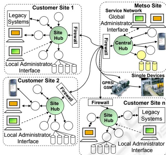
Figure 1: Site Hub network architecture.
