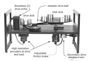
Figure 9: Mechanical system with friction.
