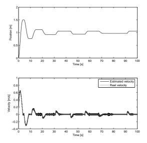
Figure 3: PID control incorporating velocity estimation from Theorem 1.
