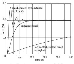
Figure 2: Effect of environmental stiffness.
