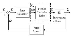
Figure 1: Robot force control.
