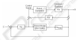
Figure 4: Robust force controller.
