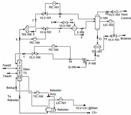
Figure 1: Distillation Column simulated in Hysys Software.
